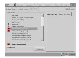
$\label{thm:condition} \mbox{Figure 7 The status display of the CMA 3000 shows the supplementary services detected on the tested line. }$
