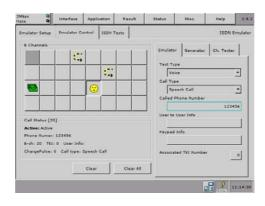
Figure 2 The status of the emulator will be presented to the user on the Emulator Control page. Calls are activated and answered in the same display.
