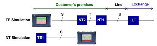
Figure 1 ISDN call emulation configurations
